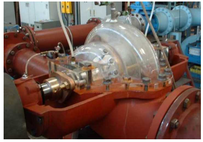
Model Pump with Transparent Casing
